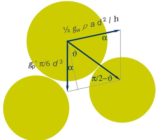
Figure 2. Two force balance of a top grain
