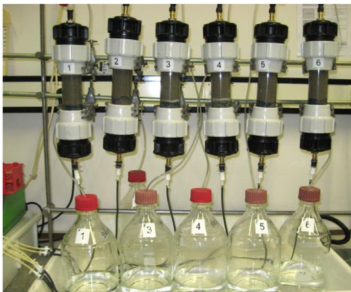
*Flow columns for determining the bonding capacity of polyaluminium chloride for phosphate*
