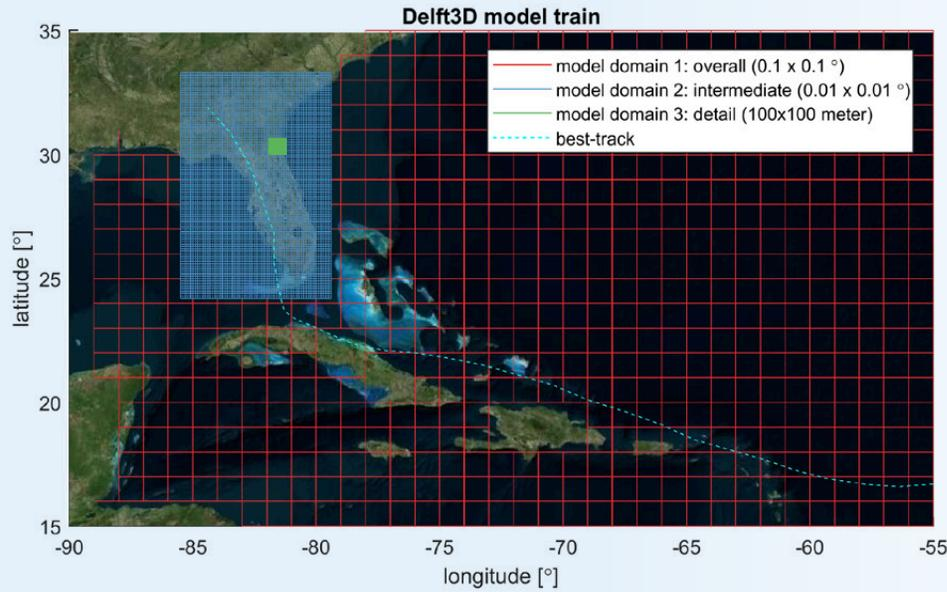
*Delft3D model train. SFINCS results were compared with the 100 m detailed model of Jacksonville*
