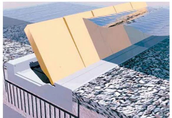
Figure 1 Schematic view of Venice flood barrier.
