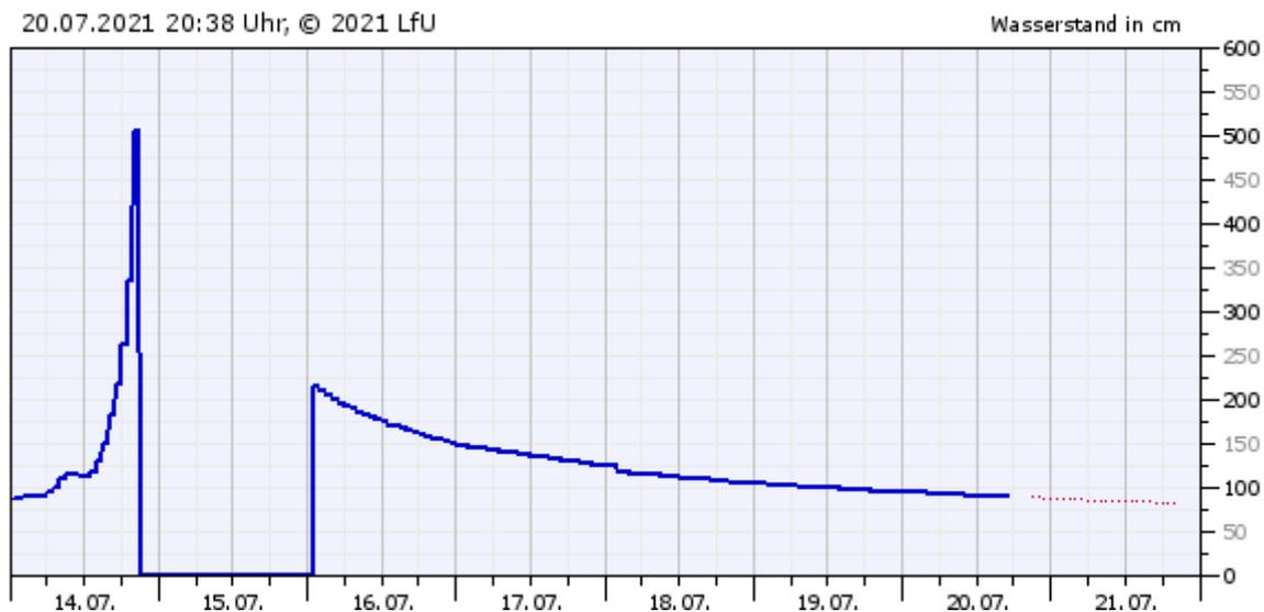
Figure 3: Measured water levels at the Altenahr monitoring station on the Ahr in Germany. Late on 14 July, the monitoring station failed. The values from 16 July onwards are values calculated using computer models for indicative purposes. The estimated water level at the high-water peak was higher than 700 cm. Source (consulted on 20/7/2021):
