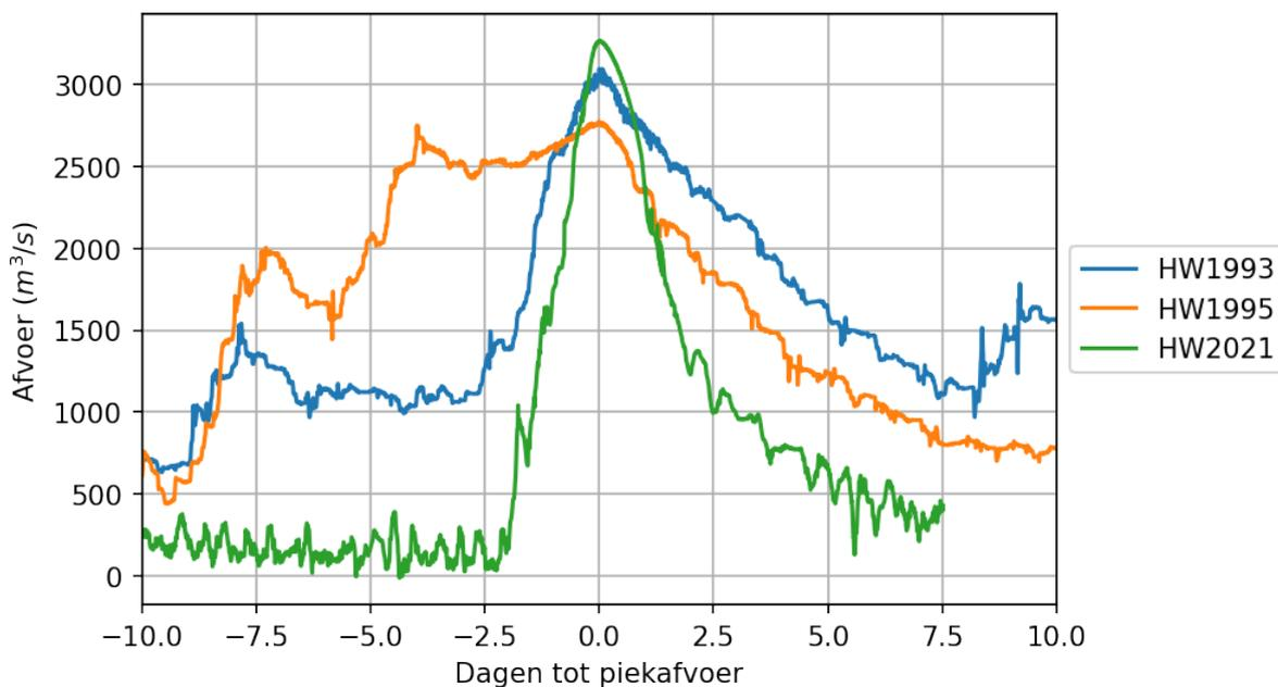
Figure: The measured discharge at the Sint Pieter monitoring station (near Maastricht) for the high water waves in 1993, 1995, and 2021
