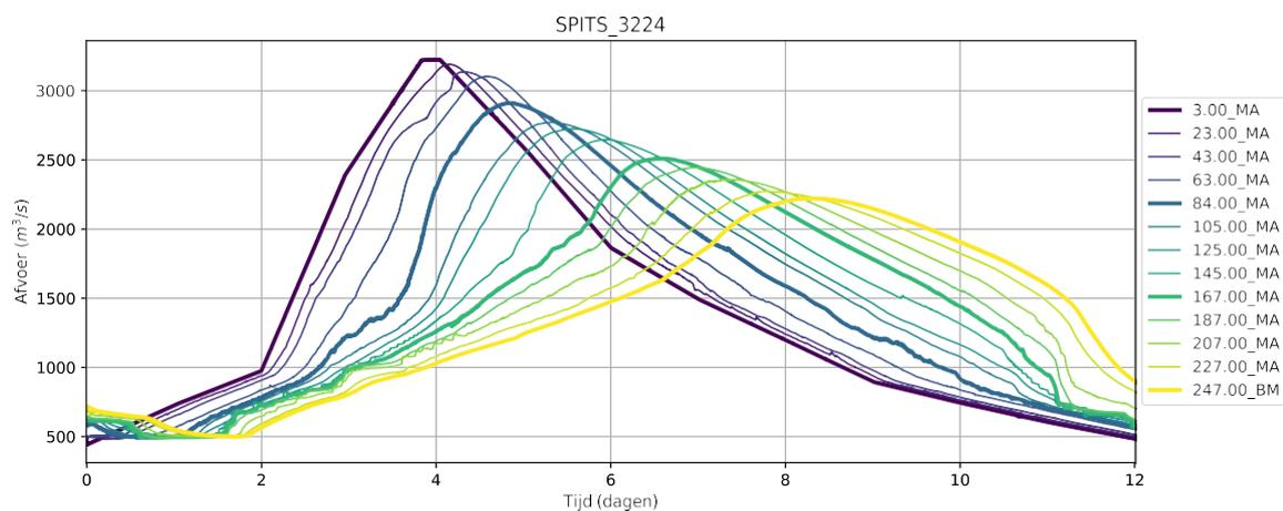
Figure: Flattening of a steep wave form as it travels along the Meuse, shown in 20-km intervals (calculated from Eijsden onwards).
