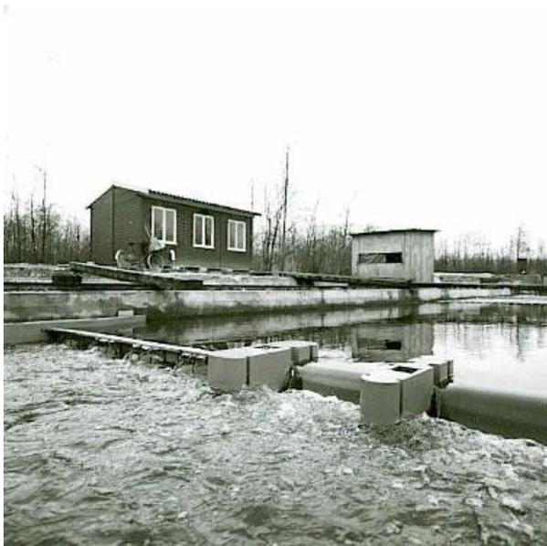
*Scale model of the weir at Sambeek; Waterloopkundig Laboratorium, 1967 (source: Deltares)*
